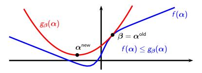
Figure: At each step, we update  $lpha\in rg \min_{lpha\in\mathcal{A}} g_eta(lpha)$
