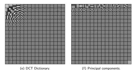
Figure: On the right, we visualize the principal components of 400 000 randomly sampled natural image patches of size  $16 \times 16$ . On the left, we display a discrete cosine transform (DCT) dictionary [Ahmed et al., 1974].
