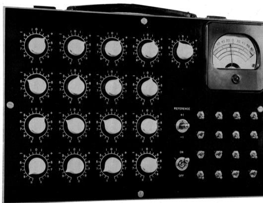
Figure: Adaline, (?): A physical device that performs least square regression using stochastic gradient descent .
