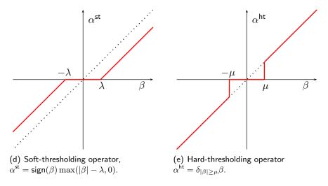
Figure: Soft- and hard-thresholding operators, which are commonly used for signal estimation with orthogonal wavelet basis.
