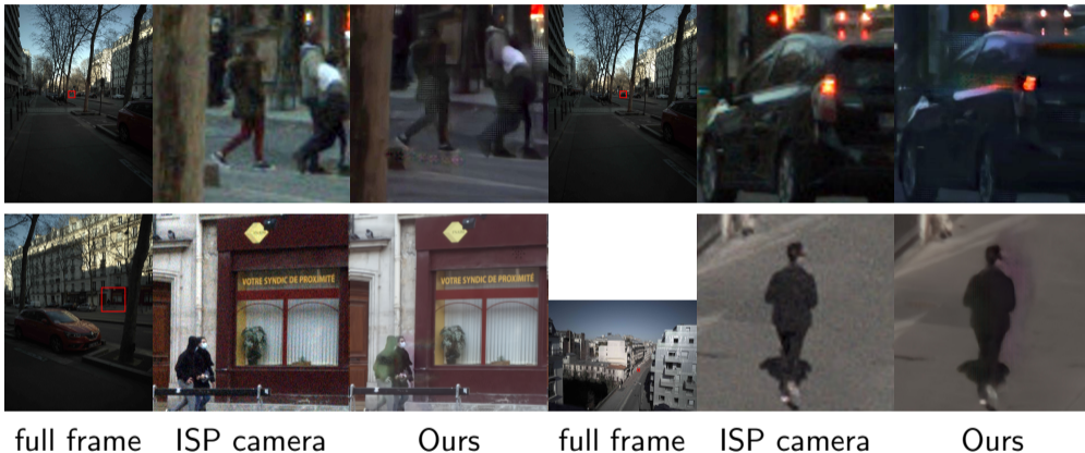
Figure: Misalignments artefacts due to moving objects in the scene. Our implementation did not handle fast moving objects and then generated visual artefacts.
