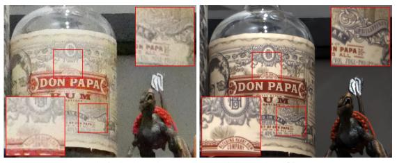
Left: high-quality jpg output of the camera ISP. Right:  $\times 4$  super-resolution, after processing a burst of 30 raw images (handheld camera).
