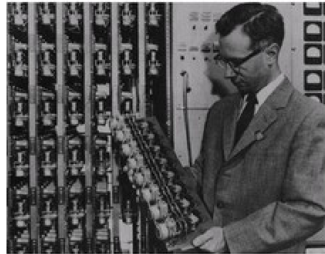
Potentiometers as weights adjusted by motors during learning
